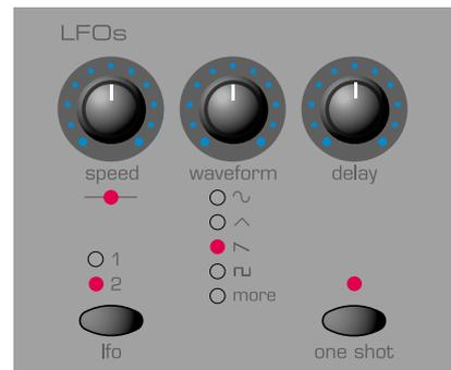
There are two independent LFOs available which may be used to modulate different synthesizer sections and run at different speeds.
